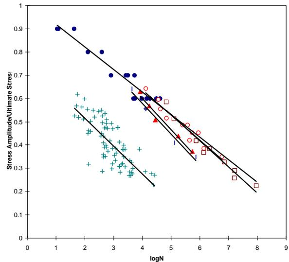
Figure 1. Comparison of normalized stress vs. cycles to failure in fatigue studies. ○, Swanson et al. (1971), human, rotating bending<sup>2</sup>; ◆, Lafferty and Raju (1979), bovine, rotating bending<sup>3</sup>; ▲, Carter et al. (1976), bovine, rotating bending<sup>4</sup>; □, King and Evans (1967), human (embalmed), rotating<sup>5</sup>; +, Carter and Caler (1981), human, uniaxial<sup>6</sup>; ●, current study, human, pure longitudinal shear.
